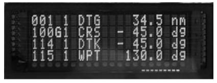
Label 001, Distance to Go (DTG); Label 100G, Selected Course (CRS); Label 114, Desired Track (DTK); Label 115, Waypoint Bearing (WPT)
