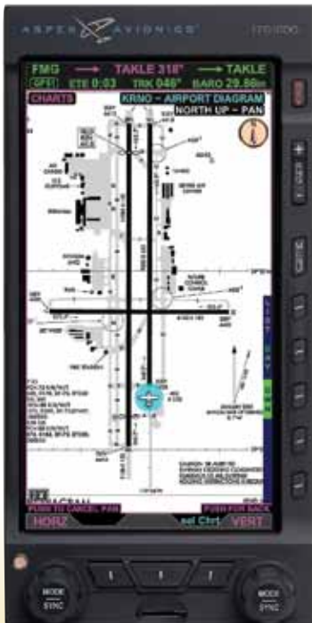
Aspen Avionics' Evolution with geo-referenced airport diagrams
