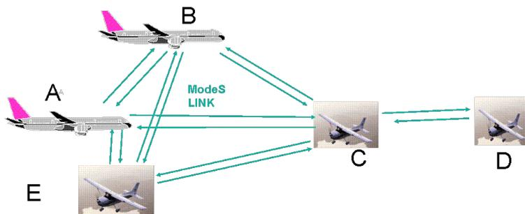
Australia has adopted a single system that allows aircraft with ADS-B IN equipment to receive ADS-B OUT from all equipped aircraft without the need for ground based translator (or “rebroadcast”) stations. In our huge country, translator stations, which are necessary to make a dual system work, would be extremely expensive. Further, translator stations on the ground add another point of failure in the relaying of air traffic data.
