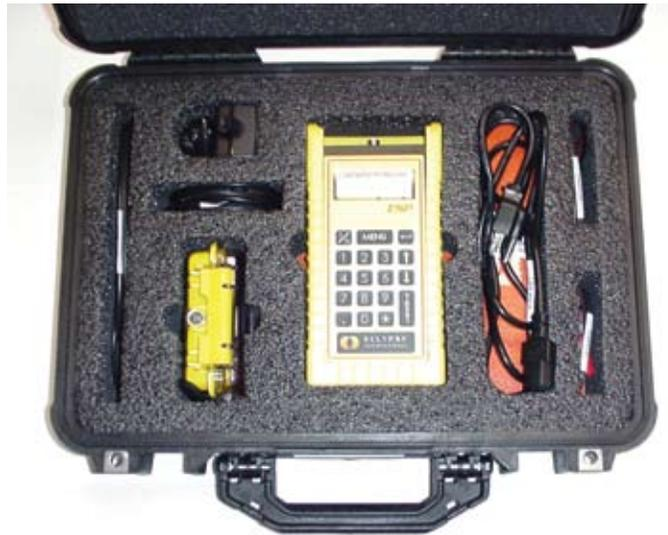
*Eclipse International Corp.'s ESP handheld unit tells the technician the distance to the fault from the point of the test leads.*
