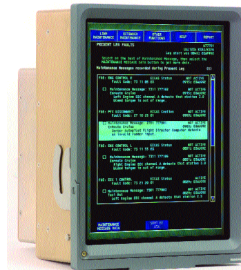
On-board diagnostics for Honeywell Primus Epic integrated avionics system display unit showing present leg faults.
