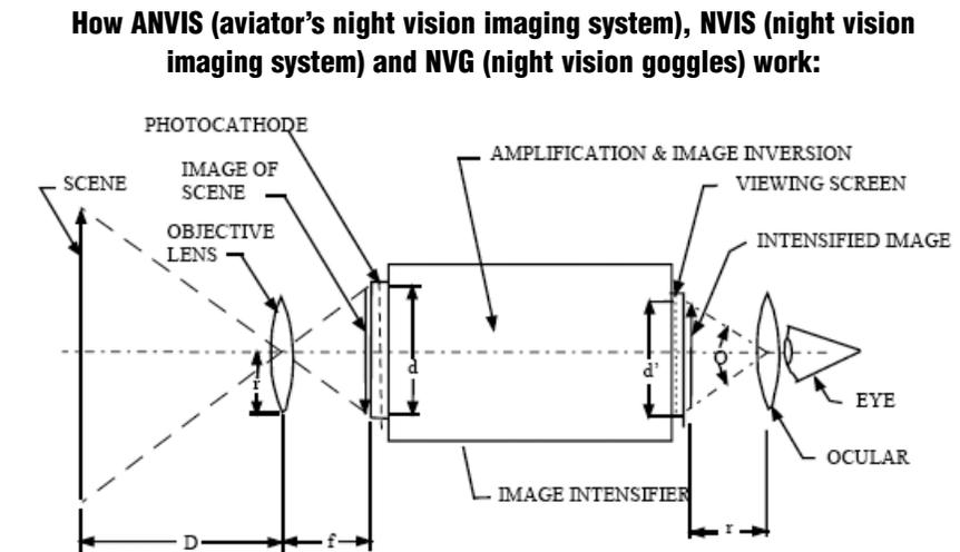
**Figure C-1. Diagram of an image intensifier.**
