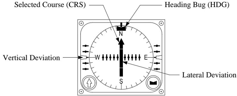
**Figure 1** Typical Horizontal Situation Indicator (HSI).
