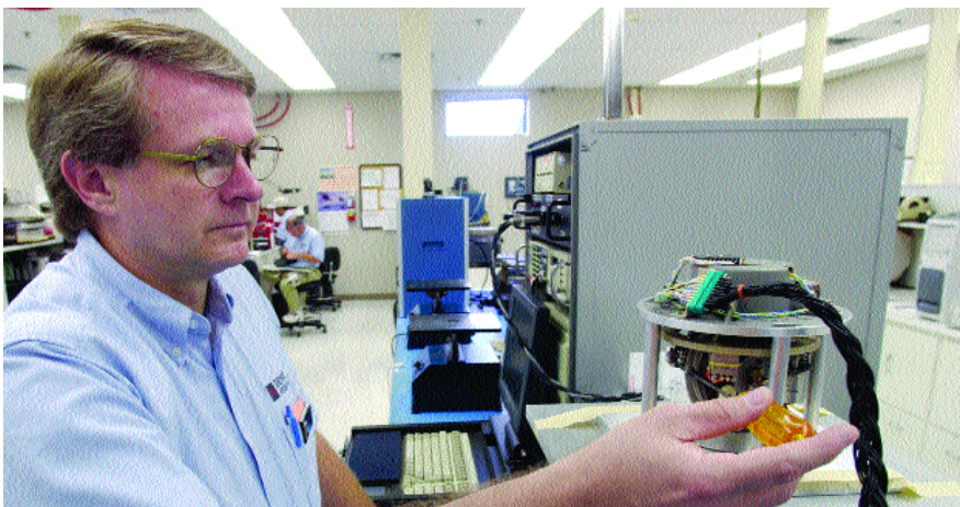
Gyro Troubleshooting Tip: It is strongly recommended that power be removed for at least 20 minutes prior to gyro handling. Photo courtesy of Duncan Aviation.
